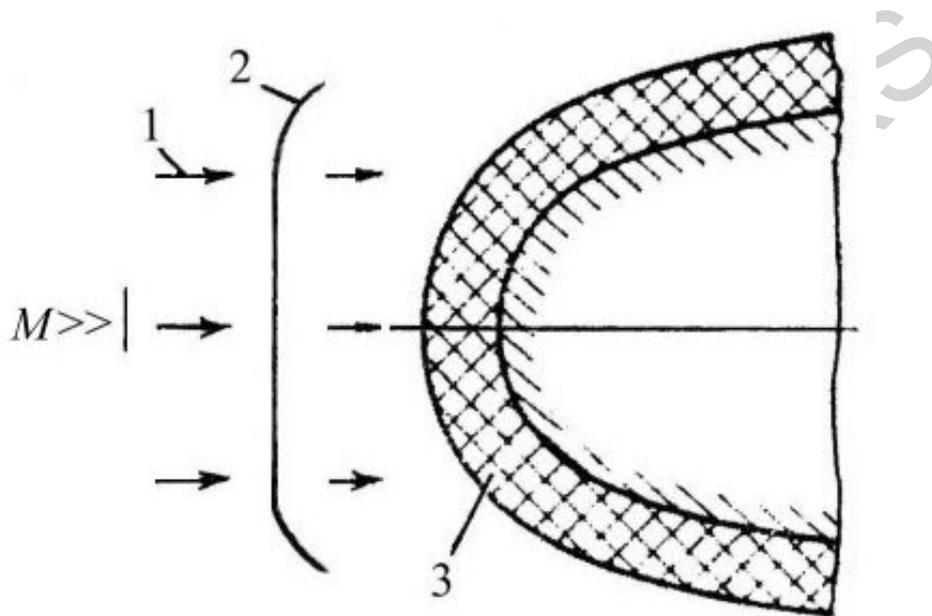
Figure 8: Schematic of the heat-protective coating of the frontal part of the flying vehicle: 1 – high-temperature gas flow; 2 – shock wave; 3 – heat-protective coating
