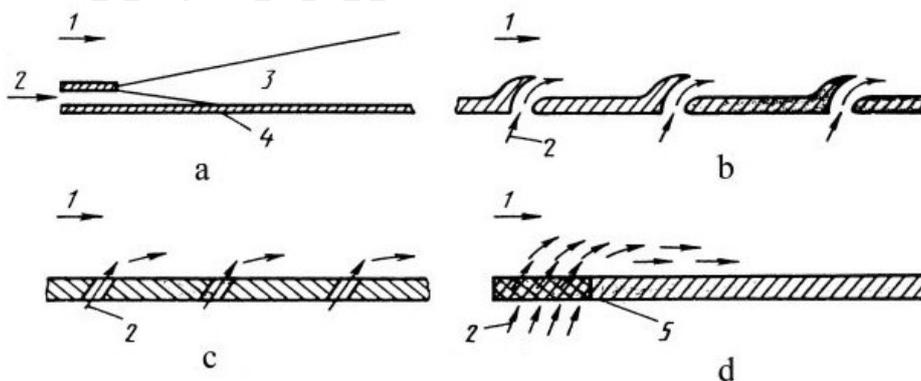
Figure 4: Schemes of coolant supply at block cooling of the surface: a – flat slit; b – system of slits; c – system of holes; d – porous insert; 1 - high-temperature gas flow; 2 – coolant; 3 – mixing region; 4 – protected surface; 5 – porous insert
