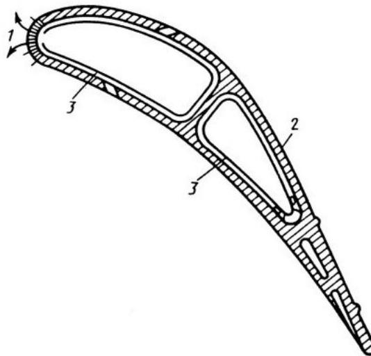
Figure 6: Scheme of convective-film cooling of the gas turbine blade: 1 – hole for coolant blowing-out; 2 – outer casing of the blade; 3 – deflectors
