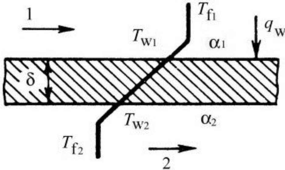
Figure 1: Convective cooling scheme: 1- high-temperature gas flow; 2 –coolant
